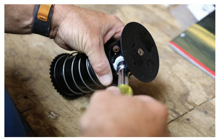
Replacing worn nozzles and adjusting them to achieve the desired coverage can save water and improve turf quality.
