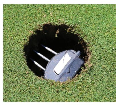
In-ground soil-moisture sensors help superintendents track moisture trends and identify thresholds for irrigation.
