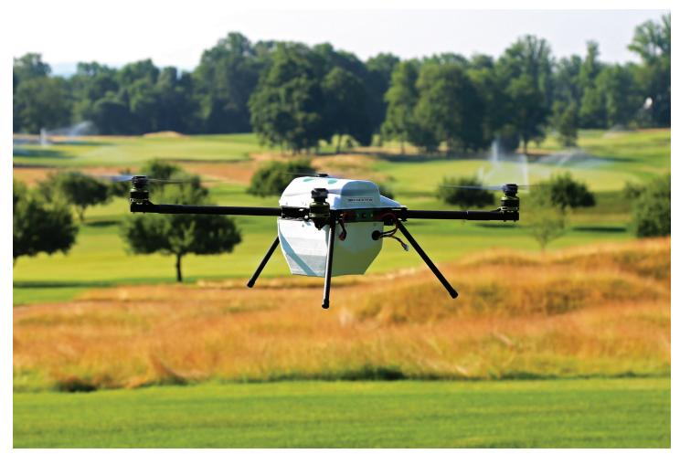
Imagery from aerial drones can identify areas of turf stress and potential irrigation issues, making scouting more efficient.
