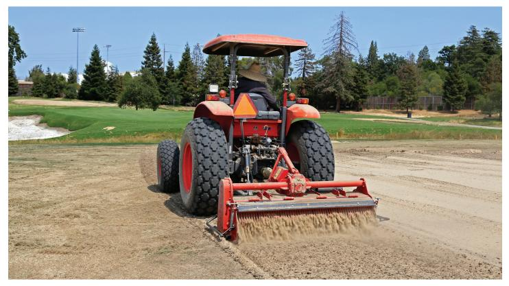
Tilling the soil before planting may be desirable, especially when planting sprigs. However, steps must be taken to protect irrigation system components and finish grading will be necessary to smooth out the surface.
