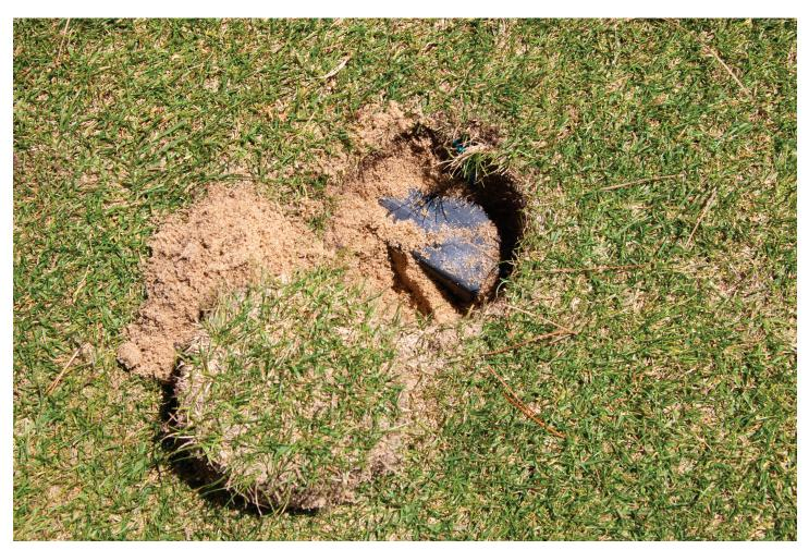
In-ground soil-moisture sensors should be installed at a consistent depth throughout the course to make measurements directly comparable.
