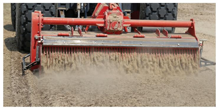
Tilling sand into heavier native soil during a renovation can improve water infiltration and salt management. Be sure to work with a physical soil testing lab to evaluate the potential performance of the mixture before moving forward.
