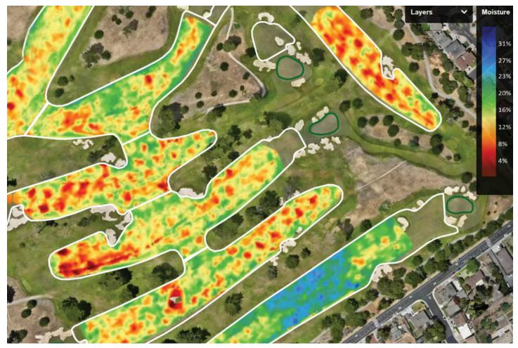
Radiometers can be mounted on mowers or other vehicles to efficiently gather and present information about soil moisture. Calibrating and assessing this information with soil-moisture sensor data is important.
