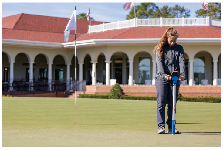
Portable soil-moisture sensors are well suited for use on putting greens because you can take many readings in a relatively small area to optimize watering. (USGA/Kyle LaFerriere)
