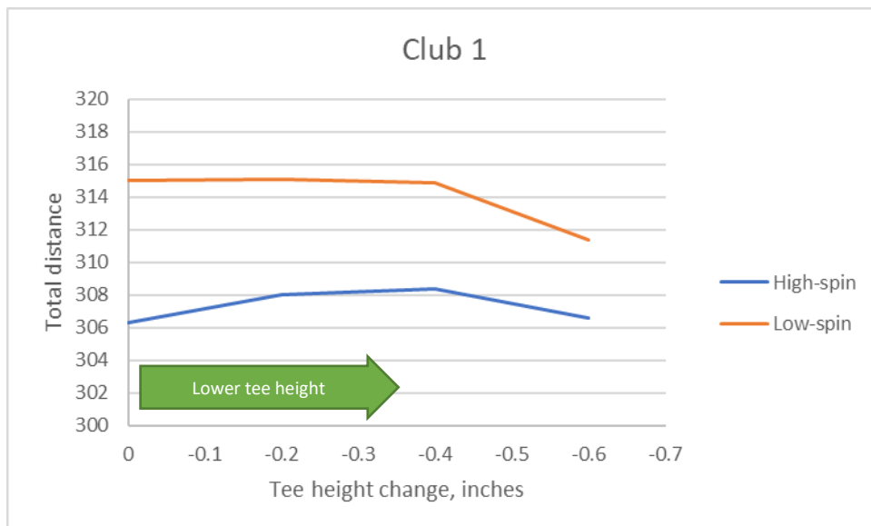
Figure 7: Total distance as a function of tee height change, club 1, two different ball types.
